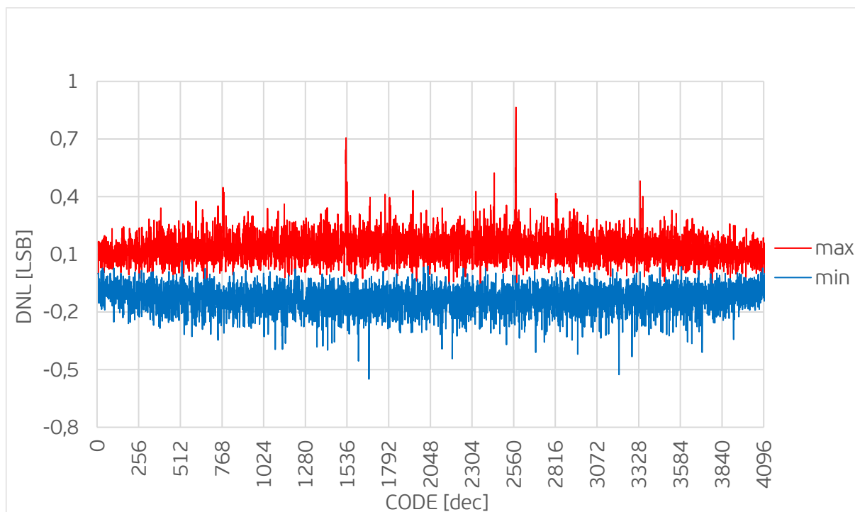
Figure 7. Minimal and maximal DNL vs output code at typical conditions ( V_{DDA} = V_{REFP} = 5\text{ V} ; V_{DDD} = 1.8\text{ V} ; T = 27^{\circ}\text{C} ; F_{CLK} = 20\text{ MHz} ; F_{in} = 1.3\text{ MHz} )
